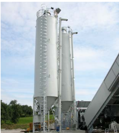
Bindemittelsilo 69 m 3 | 85 t mobil Cement silo 69 m 3 | 85 t mobile
